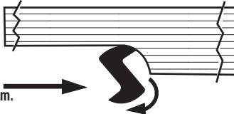
Always feed the router bit into the work piece in the same direction as the bit rotation. See diagram.
